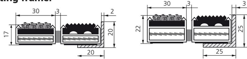
Dimensions for profiles / casting frames:
