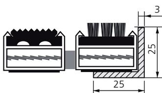
Rubber (G) and scrub cleaning (CB) in a casting frame
