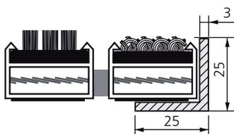
Ribbed (R) and scrub cleaning (CB) in a casting frame
